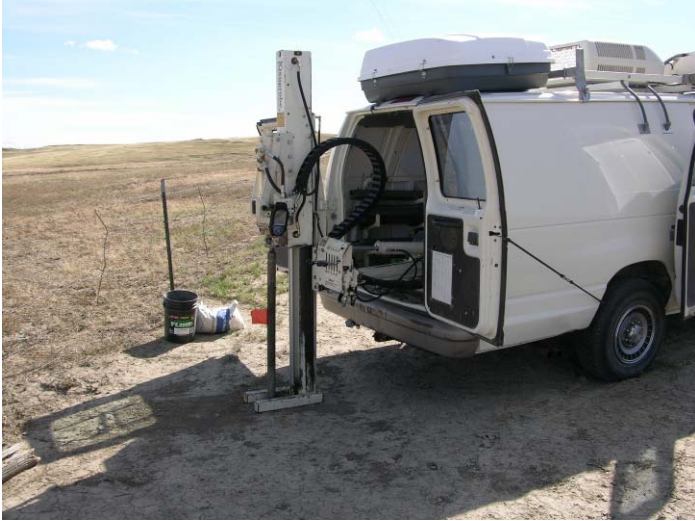
SDSM&T Geoprobe collecting soil samples in Harding County
